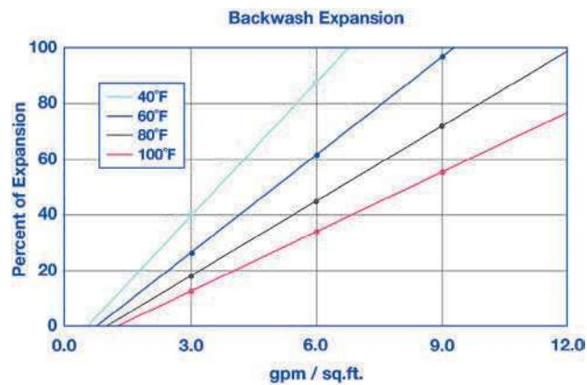
The graph above shows the expansion characteristics of ResinTech CG8 as a function of flow rate at various temperatures.
