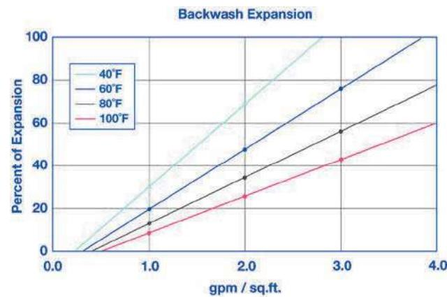
The graph above shows the expansion characteristics of ResinTech SBG1 as a function of flow rate at various temperatures.
