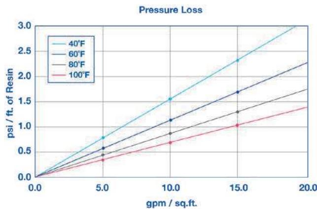
The graph above shows the expected pressure loss of ResinTech SBG1 per foot of bed depth as a function of flow rate at various temperatures.
