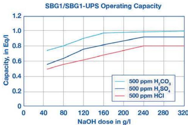
Capacity and leakage data are based on the following: 2:1 Ca:Mg ratio, 500 ppm TDS as  $\text{CaCO}_3$ , 0.2% hardness in the salt and 10% brine concentration applied co-currently through the resin over 30 minutes. No engineering downgrade has been applied.
