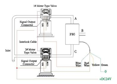
B.Assemble Two Sets of F80 to Form a Backwash System for Filter Material or Ultrafiltration Membrane
